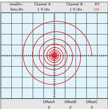
A damped LISSAJOUS diagram
