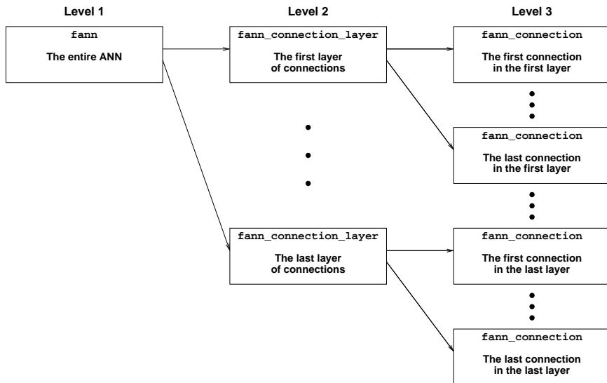
Figure 6: The three levels for the connection centered architecture. At level 3, the `fann_connection` structures consists of a weight and a pointer to each of the two connected neurons.
