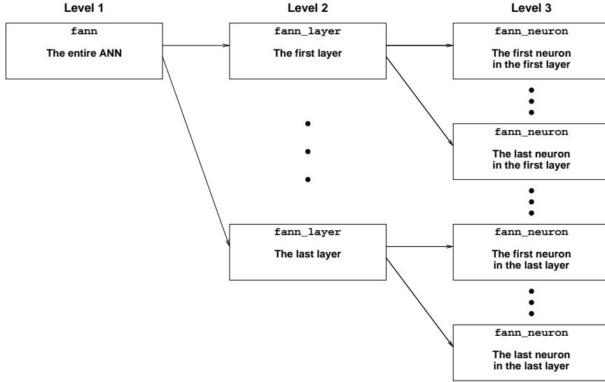
Figure 7: The three levels for the neuron centered architecture. At level 3, the **fann\_neuron** structures consists of a neuron value, a value for the number of neurons from the previous layer, connected to the neuron and two pointers. The first pointer points at the first weight for the incoming connections and the second pointer points to the first incoming connection (see figure 8).
